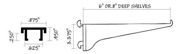
These shelf standards are designed to work with a mirror or glass backing and are at home in casinos and bars. The shelf brackets are designed to hold 6" or 8" deep material.
