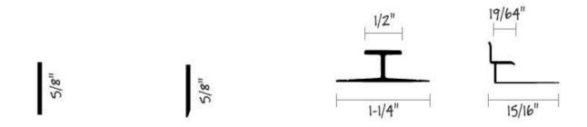
Many of the items below are designed to be used in pairs. For example, typically when hanging a mirror, you might use A718 at the top and A717 at the bottom. You slide the mirror up into the deep channel then lower it into the shallow channel.
